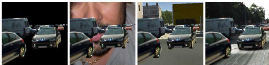
(a) Black BG AP50 = 21.5% (b) Flickr BG AP50 = 40.3% (c) Virtual KITTI BG AP50 = 47.7.3% (d) Real BG AP50 = 49.7%
